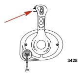
Trim switch (if equipped) - Pressing the trim switch will trim the engine up or down.
