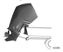
IMPORTANT: Do not rely on the power trim/tilt system or tilt support lever to maintain proper ground clearance for trailering. The outboard tilt support lever is not intended to support the outboard for trailering.
