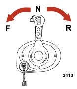
Shift lock - Pressing the shift lock allows the engine to shift. The shift lock must always be pressed when moving the control handle out of the neutral position.
