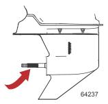
2. Lubricate the steering linkage with oil.
