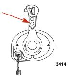
Lanyard stop switch - Turns the ignition off whenever the operator (when attached to the lanyard) moves far enough away from the operator's position to activate the switch.
