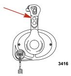
Stop/start button - Allows the boat operator to start or stop the engine without using the ignition key. The ignition key must be in the "ON" position to start the engine.
