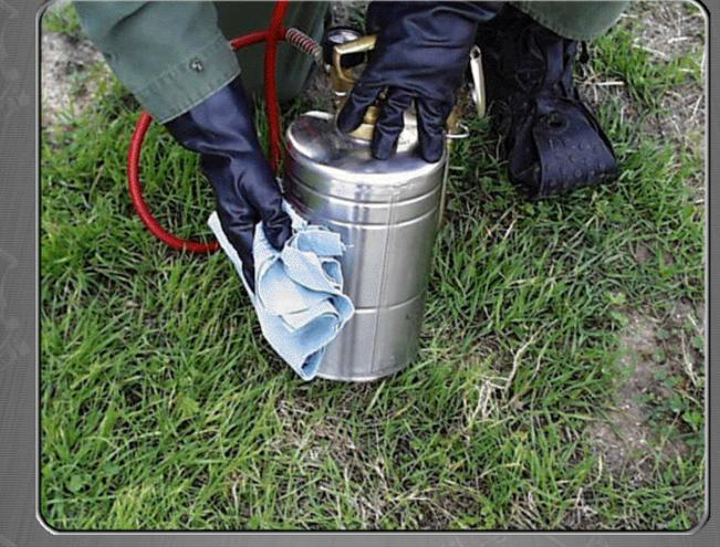
Wipe the outside of the sprayer to prevent corrosion.
